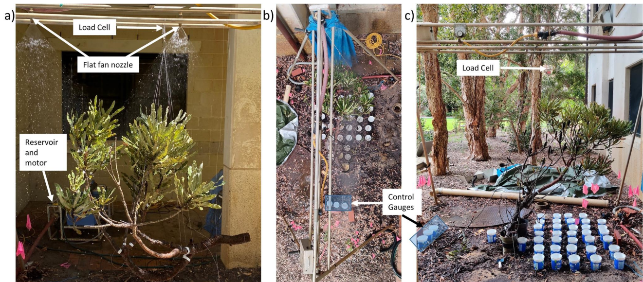
Figure 3. Rainfall simulation experiments. (a) Br1 with the rainfall simulator operational hanging from the load cell using a fishing line. Br1 did not need a gauge to measure the stemflow as all the water was being drained at the bottom of the U-bend of the branch. (b) The plan view of the rainfall simulator with the throughfall arrangement. (c) Gingin branch was monitored in the field and then was brought to the simulator, as shown in the image, with the end of the branch going into a tipping bucket rain gauge for stemflow measurement. Three throughfall buckets separated from the rest of the gauges are marked as the control buckets in (b) and (c). They are not influenced by the branch and allow comparisons between trials.
