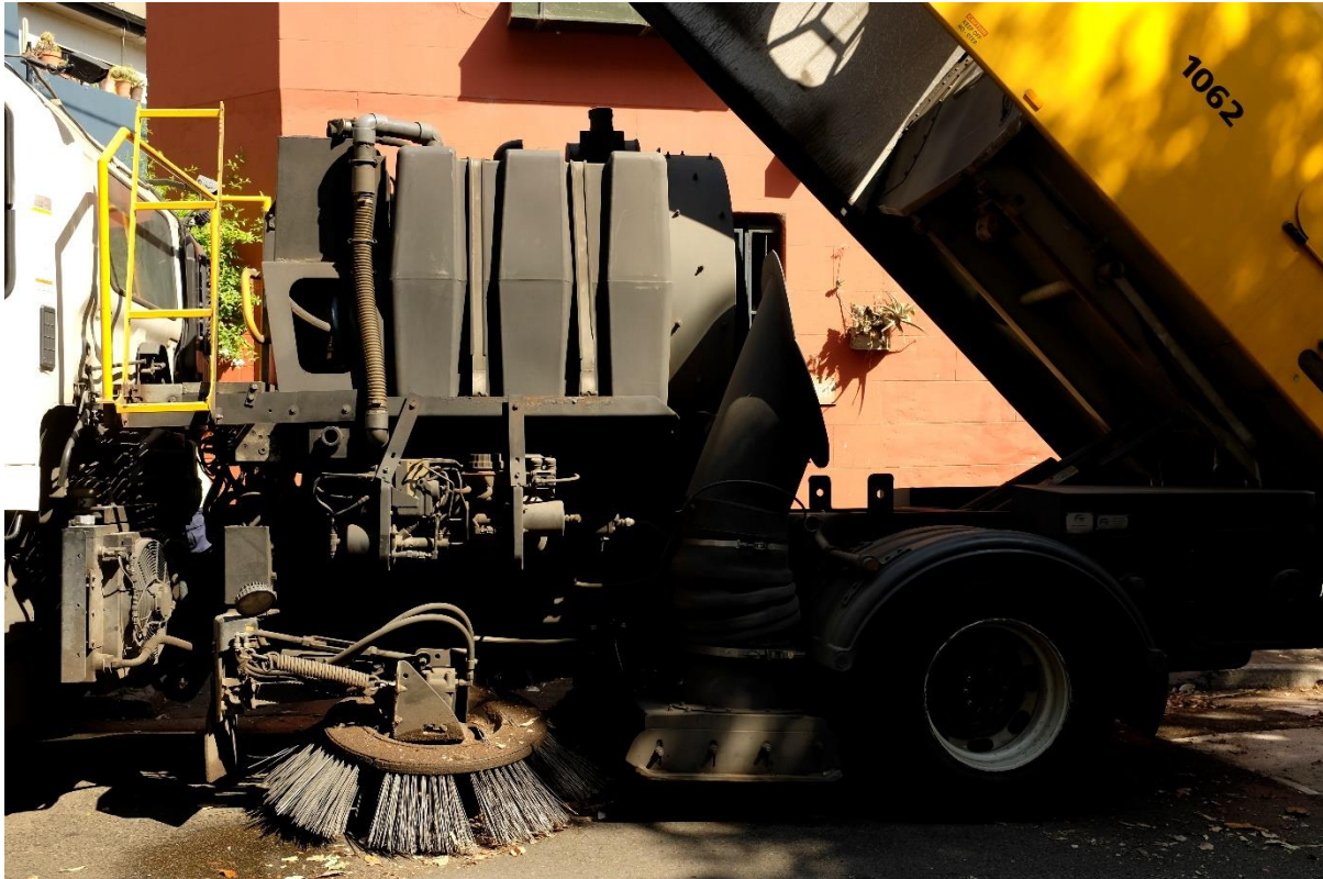
Photograph 6: Tilting the Roadway open to check for blockages
