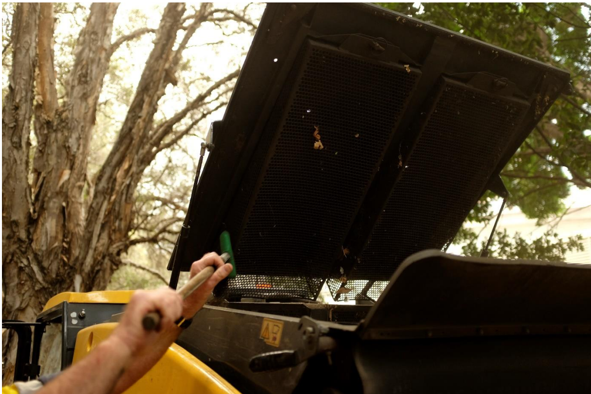
Photograph 34: Cleaning the filters
