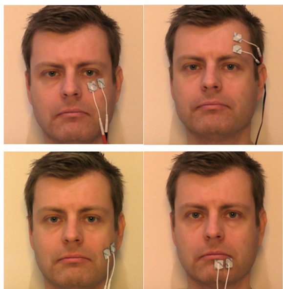
Fig. 4 Example of applying FES electrodes for external activation of facial muscles. Copyright: [128]
