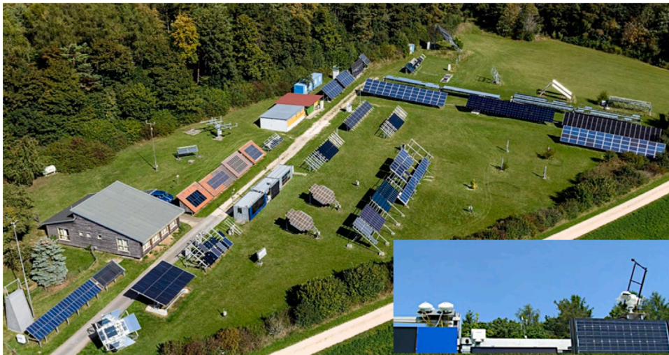
Fig. 5. Aerial view of the ZSW test site Widderstall. The insert shows part of the meteorological measurement set-up including the EKO MS-700 spectroradiometer (second from left).
