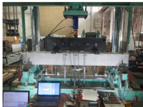
Fig. 3. Four-point flexural test setup.
