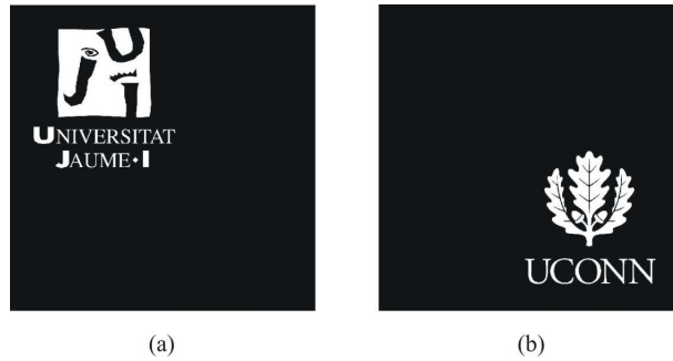
Fig. 3. Pictures of the irradiance distribution associated to the input 2D objects located at the object beam of the optical system depicted in Fig. 3. Objects (a) and (b) are assumed to be at a distance z_1 = 400\text{mm} and z_2 = 300\text{ mm} from the CCD sensor, respectively.
