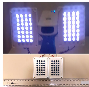
Figure 6. Final Infrared array system and its dimensions: A close-up of the mounted system (above) and actual dimensions of the Infrared array; W=100mm; H=85mm, (below) compared with 300 mm scale.
