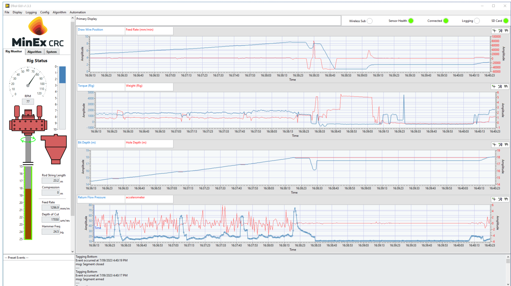
Figure 5.2: Windows-based Graphical User Interface (GUI) available to the drill operator. The algorithms developed throughout this research project were optimised for real-time applications.
