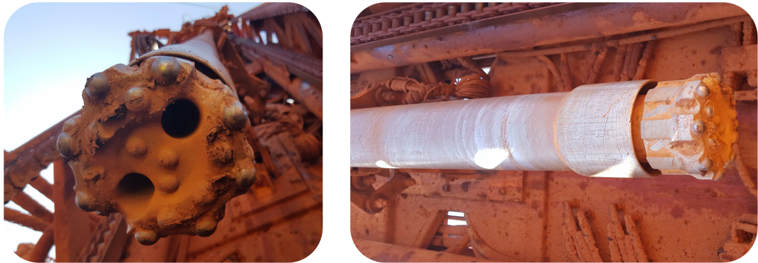
Figure 3.3: Down-the-hole hammer system utilised during the drilling operations: Schramm AD124RC hammer with a 133-millimetre ( \varnothing ) drill bit.
