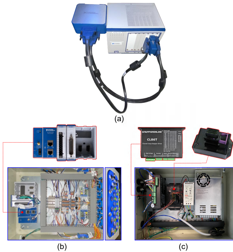
Figure 4.12: Data acquisition modules and electronics: (a) PXIe-1073 and I/O modules, (b) cDAQ-9185 and electronics circuit, and the (c) stepper motor driver and electronics.
