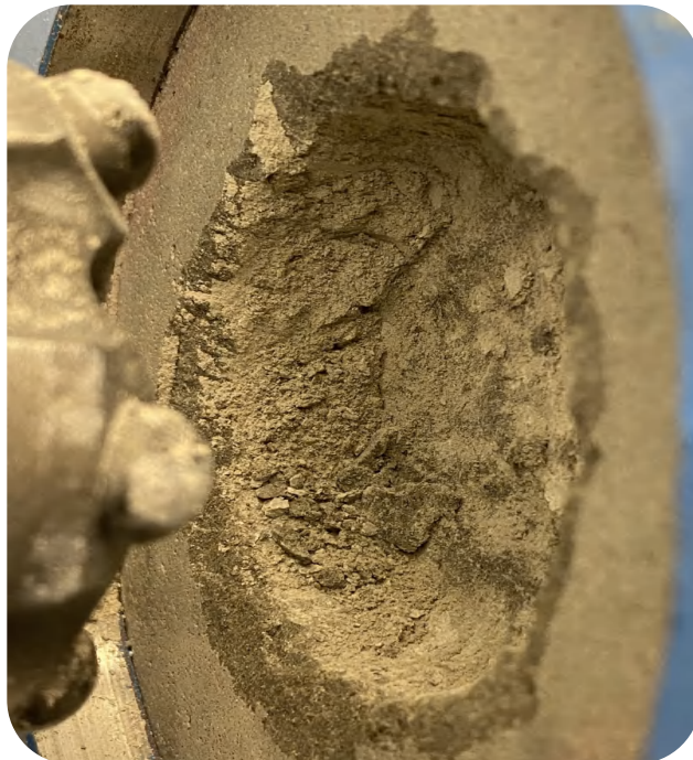
Figure 4.34: Significant cuttings and powder (dust) accumulation in the borehole. Picture taken at the end of Test 1 (impact energy=80 J, indexing angle=24°, WOB=400 kgf).
