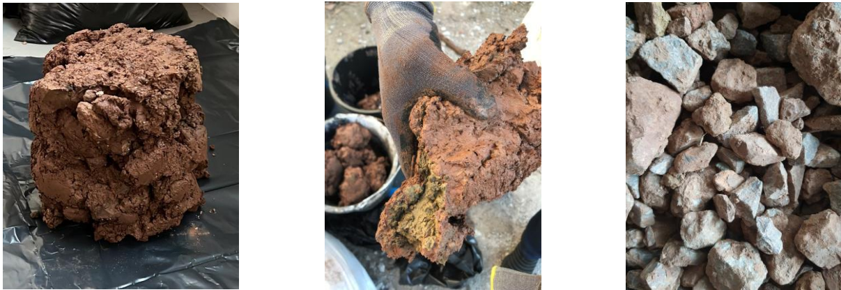
Figure 2: Delivered subsoil was not workable for extrusion, too clayey, wet and included large stones. This soil was spread and dried as chunks for a couple of days and then crushed into smaller pieces to sieve and eliminate larger stones.
