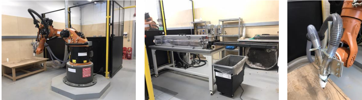
Figure 1: KUKA KR60 six axis high accuracy industrial robot, the dual extruder (Gomaa et al. [25]) and the custom fabricated steel end effector connecting 3D printed nozzle to the pressure hoses.
