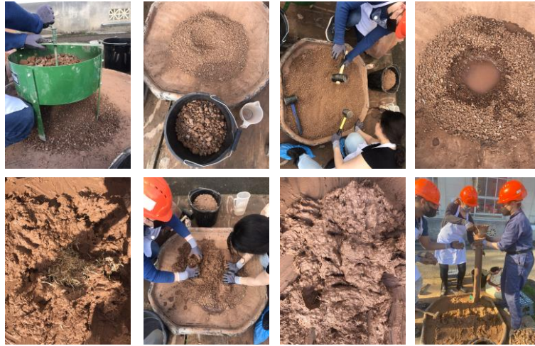
Figure 3: Soil mixing process: Sieving soil to eliminate larger stones, adding water, straw and kneading until reaching a homogenous mix. After the viscosity check, the cartridges were filled with the soil mix and sealed to keep the mix humid.
