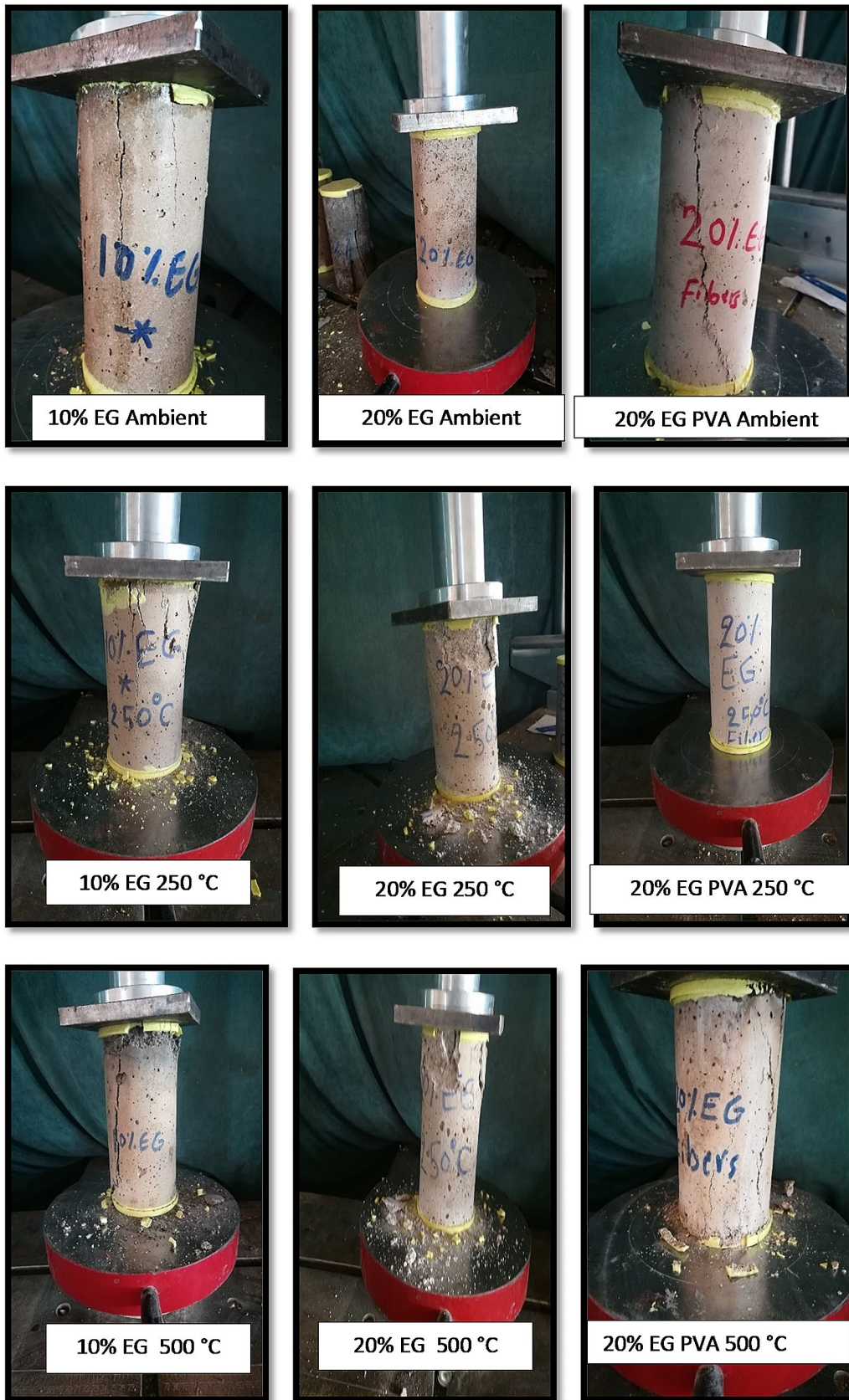
Fig. 9 Cylinder sample failure patterns at various temperatures
