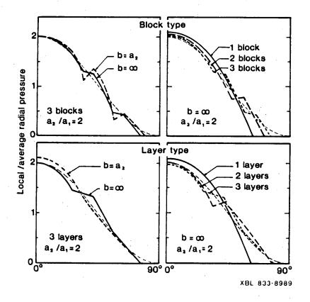
Fig. 16. Block- and layer-type coils; radial pressure distribution on outside: effects of iron radius, and number of blocks or layers.
