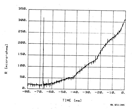
Fig. 7. Signal observed across a normal going region of the "north pole" of D-8A during a quench.
