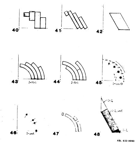
Figs. 21-48. Cross sections of windings for accelerator dipoles. The details of each configuration are described in the text.
