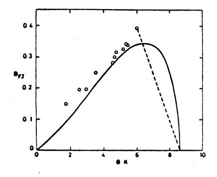
Fig. 5. Experimental measurements of the flux jumping field in NbTi compared with the theoretical value.
