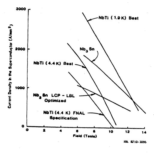
Fig. 49. Critical current density as a function of magnetic field in commercially available superconductors.
