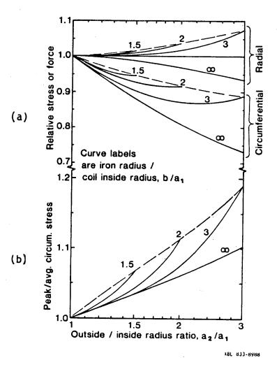
Fig. 14. Thick cos θ coil. Upper curves are max. radial stress on outside of coil and total circum. force normalized to values for thin coil producing same field. Lower curves are peak-to-average circum. stress ratio.
