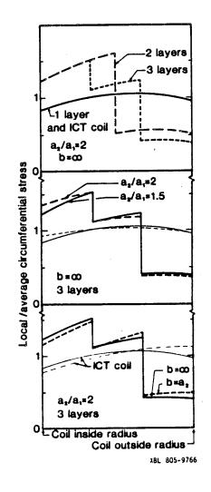
Fig. 17. Layer-type coils: circumferential stress distribution at  $\theta = 0$ , effects of number of layers, coil thickness, and iron radius.
