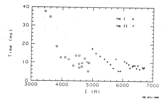
Fig. 8b. Transverse quench propagation: transit time from 1st to 2nd turn vs. current.
