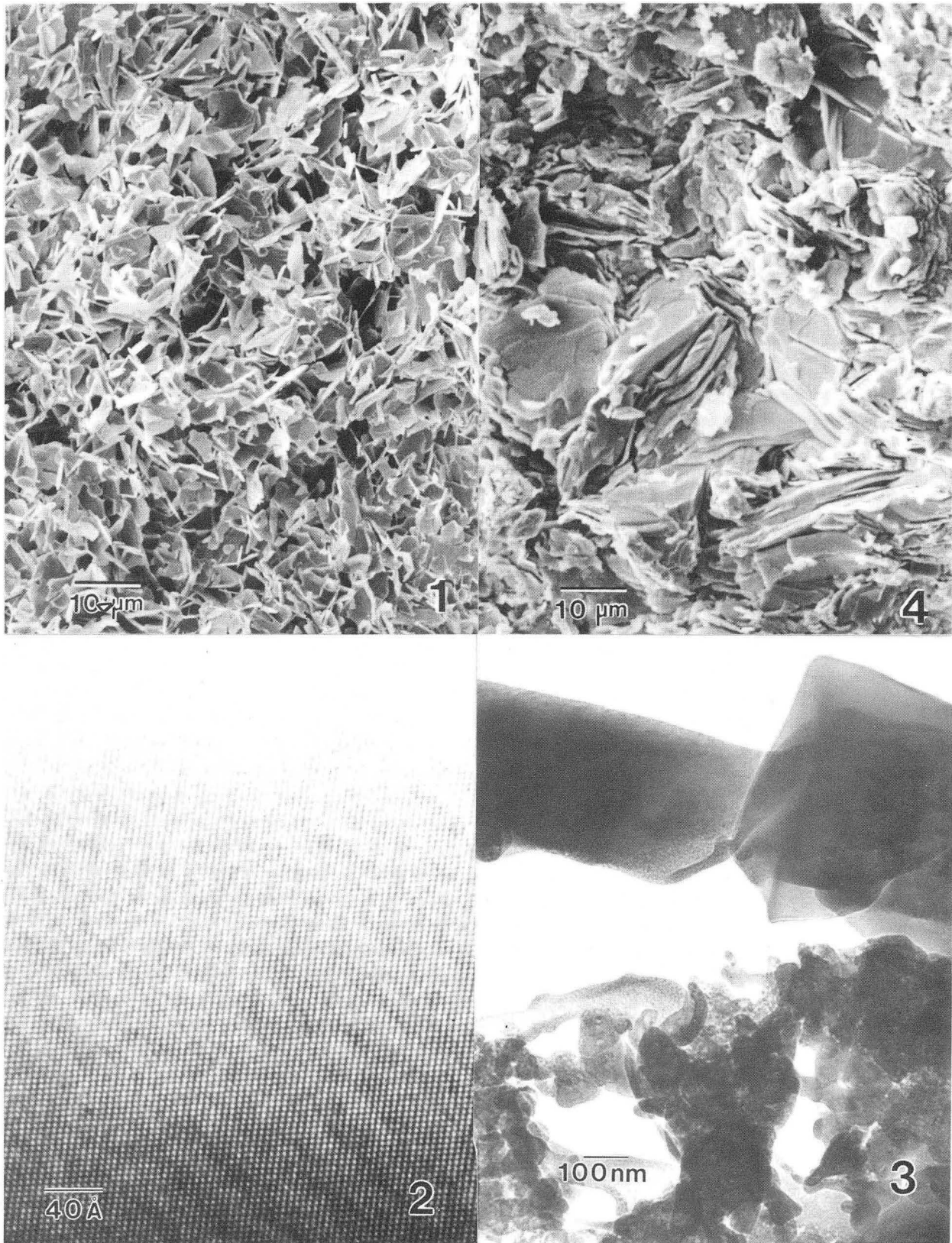
FIG. 1. -- Scanning electron image of porous microstructure in sintered pellet of BiCaSrCuO. FIG. 2. -- High Resolution TEM image from crushed specimen, showing (001) cleavage. FIG. 3. -- TEM image of ion milling damage in porous material. FIG. 4. -- Scanning electron image of sintered BiCaSrCuO pellet with additional processing.
