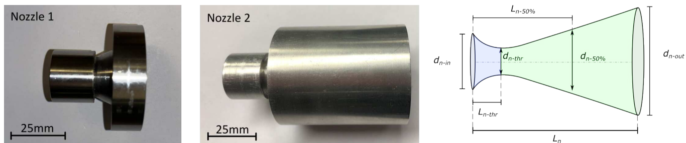
FIG. 3. Picture of Nozzle 1 (left) and Nozzle 2 (middle) used in experiments and a schematic of an arbitrary nozzle (right) profile with the main characterising dimensions as shown in Table I. Blue coloured section refers to the converging section and green coloured refers to the diverging section. Dimensions for nozzles used in this study can be seen in Table I.
