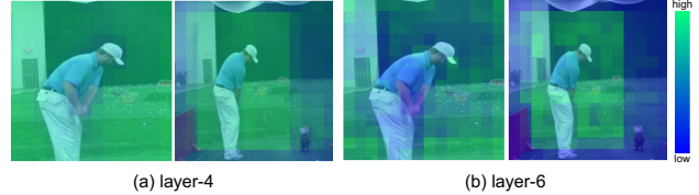
Figure 5. Visualization of the temporal matching function f_{tem} on an example frame pair. A large value of f_{tem}(i) indicates that the i -th pixel matches well to a pixel in the other frame.
