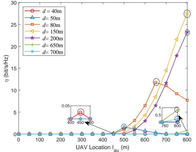
Fig. 3. The ECT  $\eta$  versus the locations of UAV and Willie.
