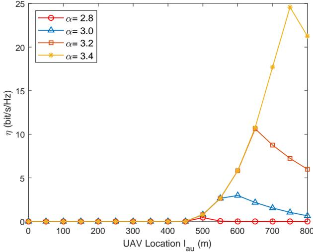
Fig. 4. The ECT  $\eta$  versus the path-loss exponent from Alice to Willie  $\alpha$ .
