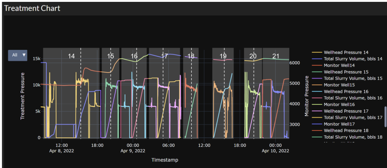
Figure 103: Example treatment stages with the volume to first response occurrence time annotated for each stage.
