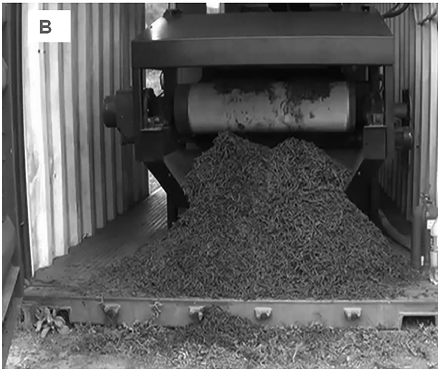
FIGURE 6.5 Schematic diagram of the LaDePa process (A) and the pellets that are produced (B) (Mirara et al., 2020).
