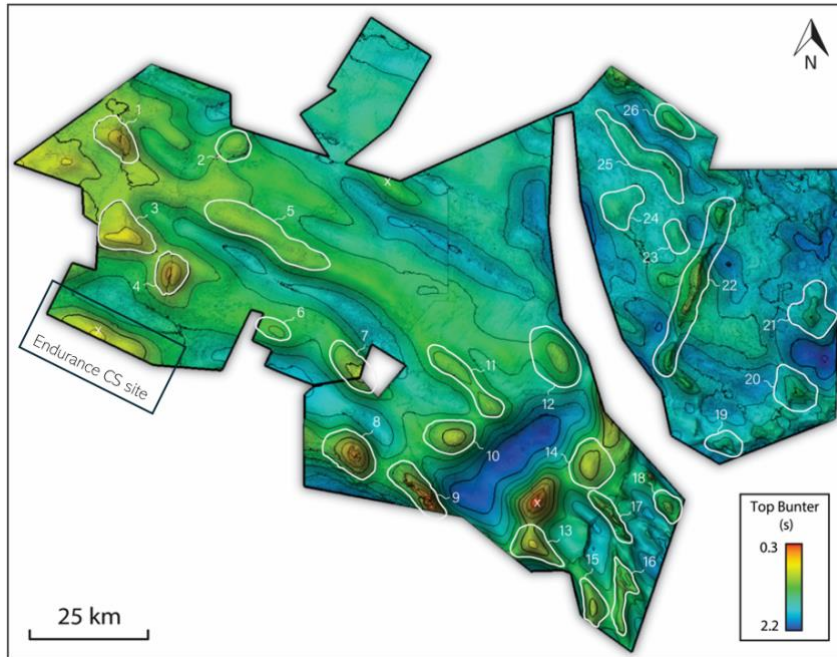
Figure 4 - Map of the top surface of the Bunter Reservoir showing the salt domes studied (white contours). Topography of the top Bunter surface displayed in time units (seconds).
