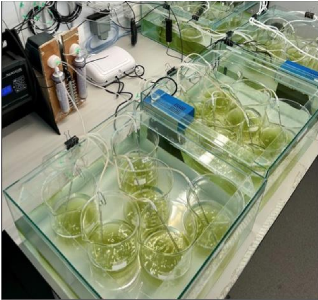
Figure 10. Experimental setup with phytoplankton culture containers (microcosms) used to test the effects of CO 2 leakage and warming on phytoplankton communities.
