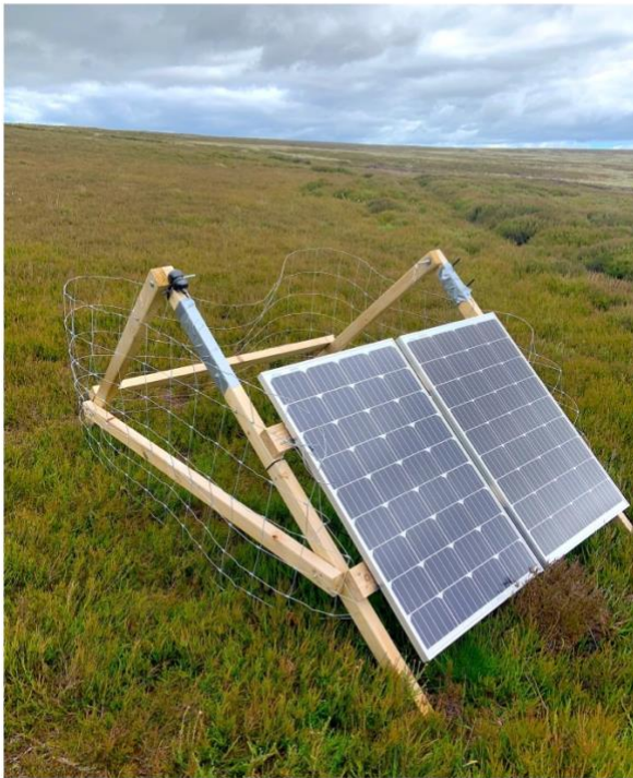
Figure 6 - One of the eight seismic stations that form our array. The seismometer is buried up to 1m deep with only the solar panel, which powers the system, and telemetry equipment, left above ground. [Source: Joseph Asplet, 2024]
