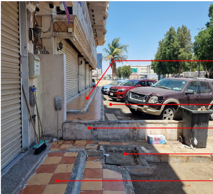
Figure 6-38. Flagged sidewalk design and obstruction issues.
