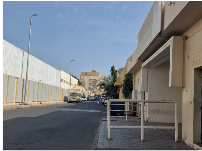
Figure 6-26. Placement of protective fences to prevent cars from hitting students on their way in/out of schools as well as parking. Simultaneously, these fences block the movement of pedestrians on sidewalks (when available).
