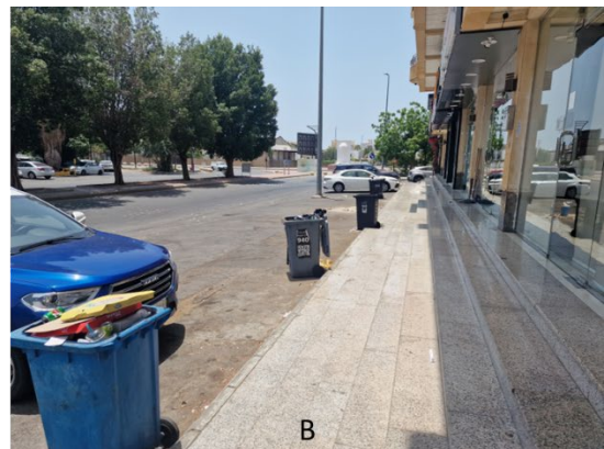
Figure 6-36. Trash bins in both A & B are unaccounted for in the design of sidewalks, which obstruct pedestrian movement in cases such as "A".
