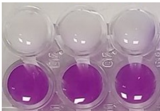
Figure 3.7. LcpK30 colourimetric analysis. After incubating with Schiff's reagent, the natural rubber degradation products with aldehyde terminal ends reacted with Schiff's reagent to give a magenta colour. The reagent was added to the reaction mixture in a 1:1 ratio.
