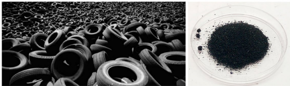
Figure 1.6. Crumb rubber made from tire waste. 56,57
