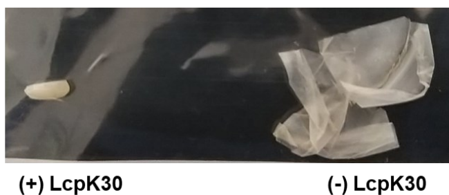
Figure 4.16. The physical morphology changes of the treated and non-treated h -IR-100K films.
