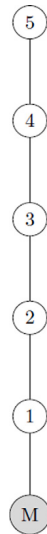
Fig. 4. Attributed graph for the Piper Tomahawk aircraft wing. White and grey circles denote structural and boundary nodes respectively.
