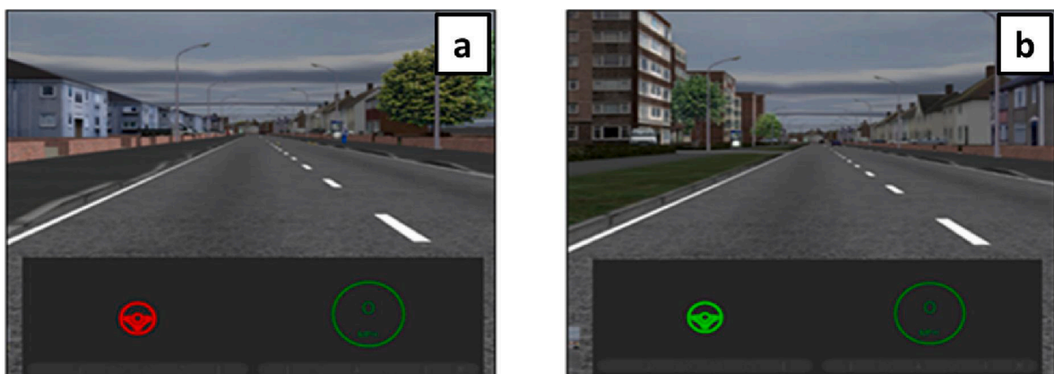
Fig. 1. HMI Interface on the dashboard: (a) when automation was disengaged; (b) Automation was engaged (from Radhakrishnan et al., 2022).
