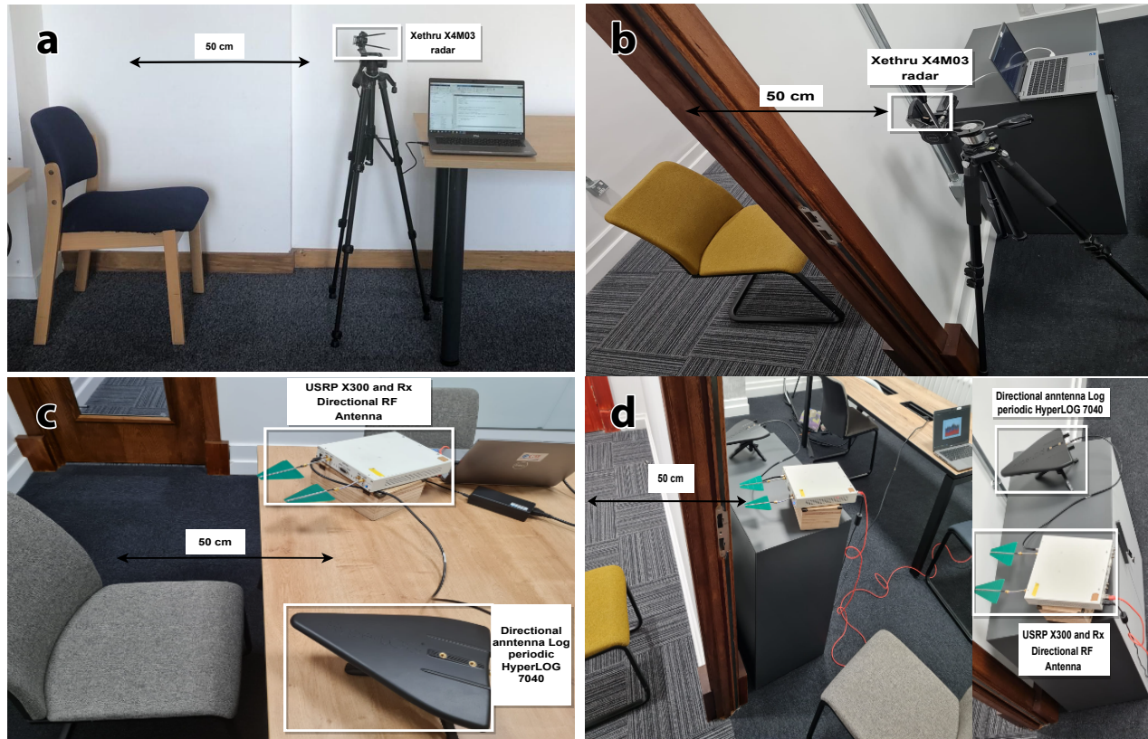
Figure 3. Head movements activity with their representation in Wi-Fi and radar signal. (a) An experimental setup of the radar signal without wall. (b) An experimental setup of radar signal through a wall. (c) An experimental setup of Wi-Fi signal without wall. (d) An experimental setup of Wi-Fi signal through wall.
