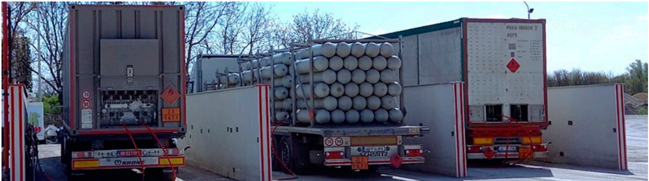
Figure 3. Considered semi-trailers with MEGC bodies (left and right) and battery bodies (middle).
