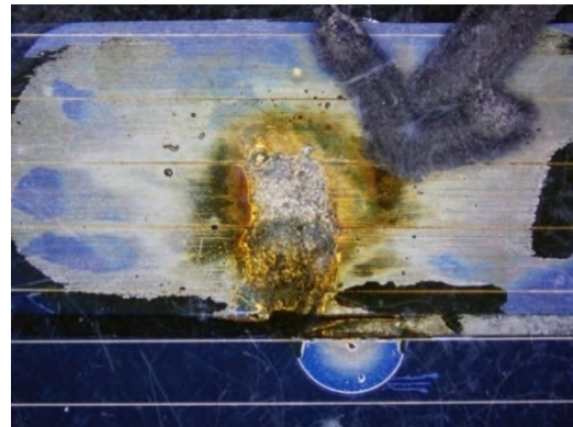
Figure 2. Solar cell, damage appearance, magnification 10x, industrial light microscope.
