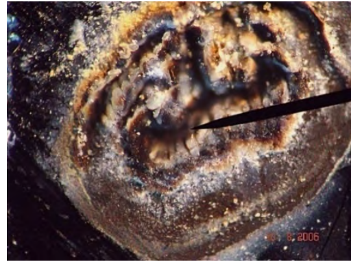
Figure 6. Pure Si, Point P1 (uz3), damage appearance, magnification 10x, light microscope.
