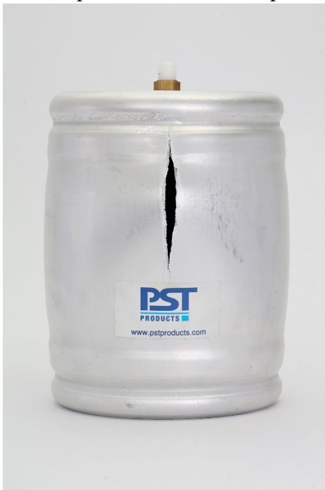
Figure 5: EMPT-cripped vessel after burst pressure test
