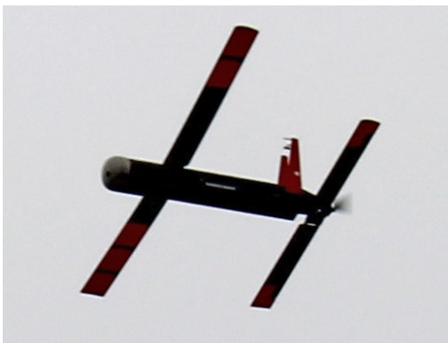
Figure 4.3: Tandem-wing configuration: Raytheon Coyote (public domain, cropped) (NOAA, 2016). Wingspan: 1.47 m (Streetly & Bernadi, 2018).
