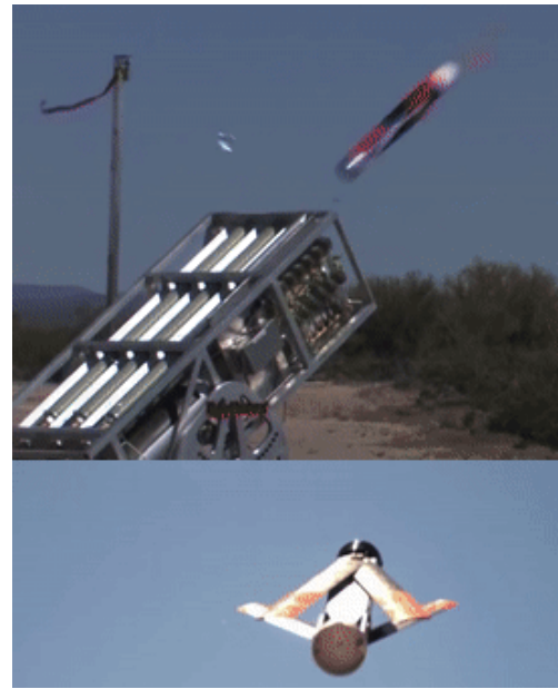
Figure 4.11: Raytheon Coyote launched from low-cost UAV swarming technology (LOCUST) launcher (public domain, cropped) (Smalley, 2015).
