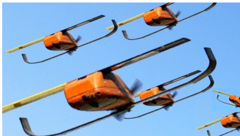
Figure 5.3: SCO Perdix with swarm-flight capability (public domain) (Dyndal et al., 2017).
