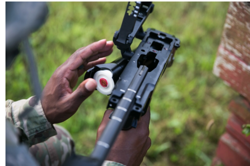
(b) Drone-40 inserted into M320 40 mm grenade launcher.
