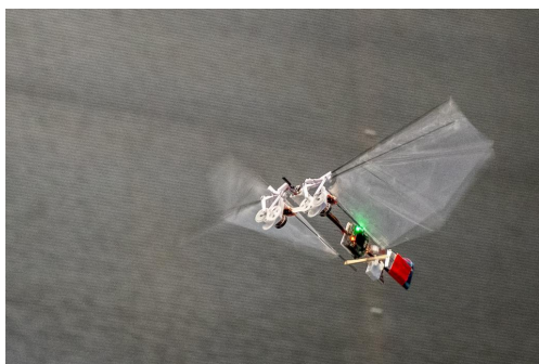
Figure 4.8: DelFly Nimble . Wingspan: 33 cm (public domain) (MAVLab TU Delft, 2018; de Croon et al., 2016).
