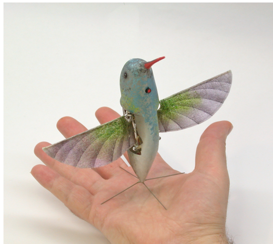
Figure 5.1: AeroVironment Nano Hummingbird prototype with right body panel removed. Total mass: 19.0 g, Flap rate: 30 Hz, wingspan: 16.5 cm, speed: from hover to 6.7 m/s, endurance: 4.0 min (Keennon et al., 2012, p. 4, fig. 11, table 2). Image source: (AeroVironment, 2021a) ((C) AeroVironment, reprinted by permission).
