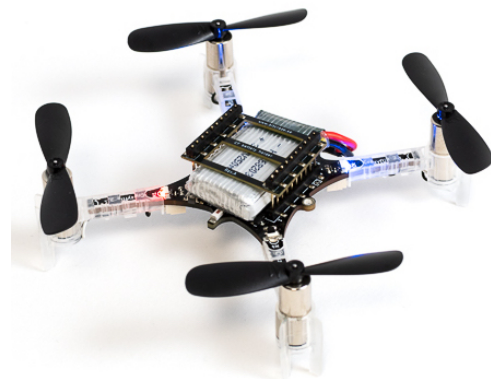
Figure 4.6: Quadrotor Bitcraze Crazyflie 2.1 . Width (motor-to-motor and including motor mount feet): 9.2 cm ((C) Bitcraze, reprinted by permission) (Bitcraze, 2020).
