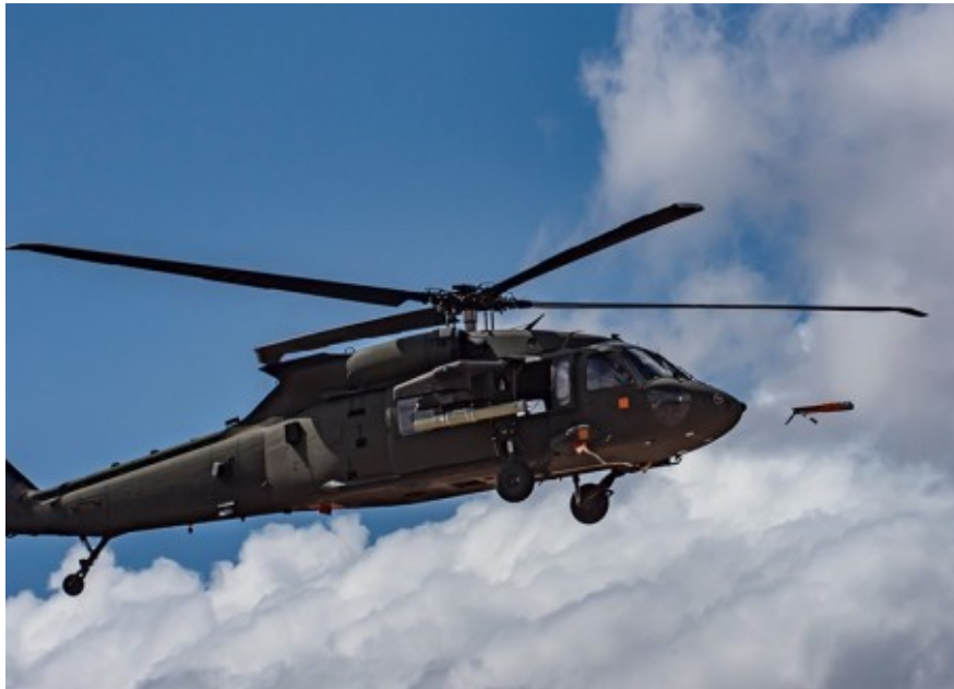
Figure 5.4: UH-60 Black Hawk launching a Area-I ALTIUS-600 UAV during flight (public domain) (PEO Aviation, 2020).
