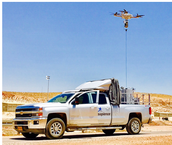
Figure 4.13: Sky Sapience HoverMast tethered to power supply unit transported on a pick-up truck ((C) SkySapience, reprinted by permission) (Sky Sapience, 2020).
