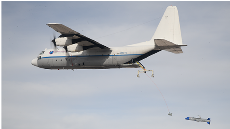
Figure 5.2: Third flight of the Dynetics X-61A Gremlins Air Vehicle launched from a customized Lockheed C-130 Hercules (public domain) (DARPA, 2020a).
