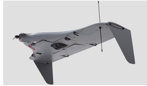
Figure 4.2: Flying wing with tractor propeller: Spaitech Sparrow . Wingspan: 0.98 m ((C) Spaitech, reprinted by permission) (Spaitech, 2019).
