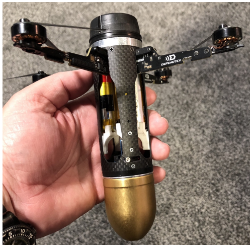
(a) After launch, the rotor arms extract and the UAV acts as a quadcopter.
