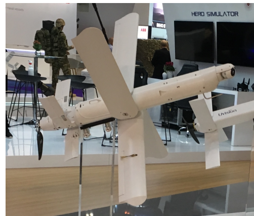
Figure 4.4: Custom wing configuration: UVision HERO-30 (public domain, cropped) (Swadim, 2019). Exact size unknown.
