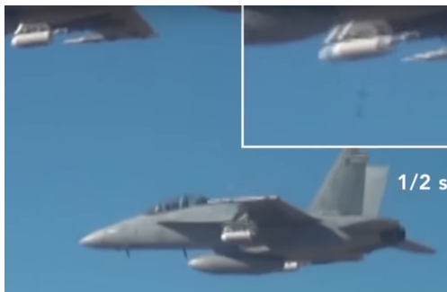
Figure 4.14: Swarm deployment from three F/A-18 Super Hornets in October 2016 (public domain) (TIME, 2018).
