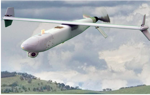
Figure 4.1: Conventional fixed-wing configuration: IAI GreenDragon ((C) IAI, reprinted by permission) (IAI, 2019a). Wingspan: 1.7 m (IAI, 2019b).
