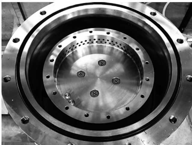
FIGURE 2 Perforated bowl-type rotor used in RPB
