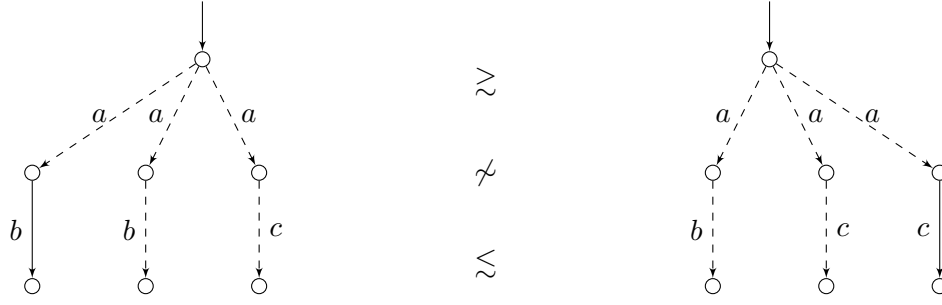
Figure 6.3: Example of two MTSs that modally refine each other, however which are not bisimilar when may and must transitions are viewed as different entities.
