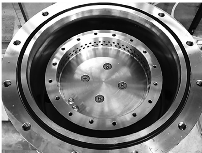
Figure 2 Perforated bowl-type rotor used in RPB.
