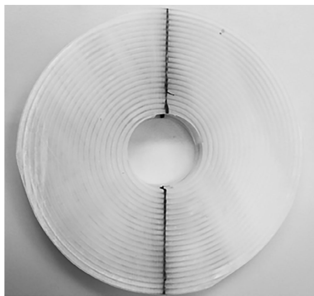
Figure 3 3D printed spiral packing used in the experimental study.
