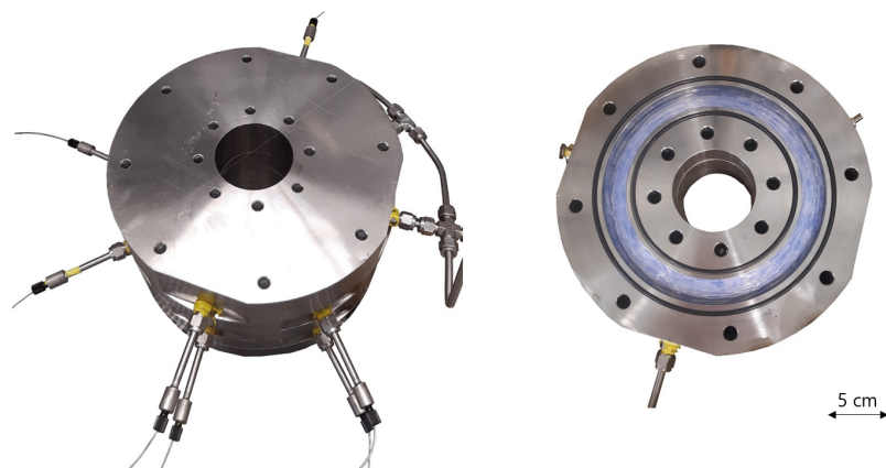
Figure 2.12. Left: Main capillary reactor. This steel housing is electrically heated and represents the reaction zone. The steel housing is divided into four individual elements that are stacked together. A single element with an inner capillary is shown on the right.
