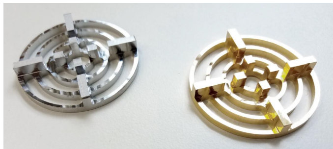
Figure D.2. Anode insert. Left: Stainless steel; Right: Gold-plated stainless steel.
