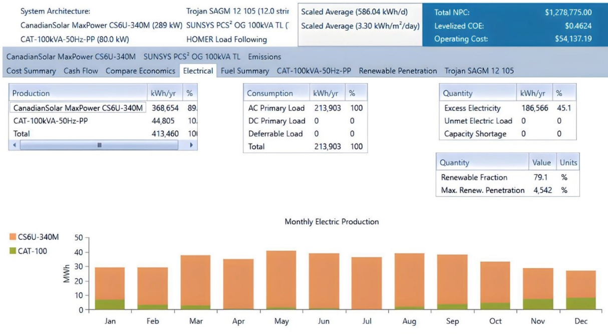
Figure 2.9: Monthly Electricity Production by PV & Gen (10% Less Load & 10% more Solar Insolation Level)
