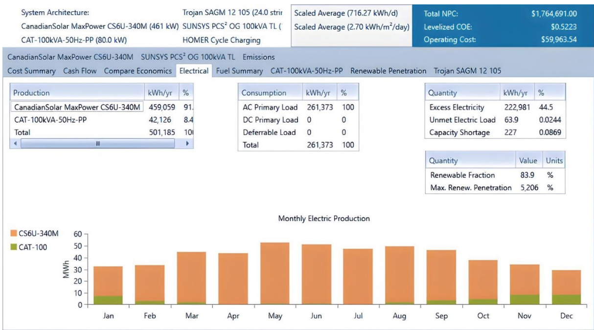
Figure 2.10: Monthly Electricity Production by PV & Gen (10% more Load & 10% less Solar Insolation Level)
