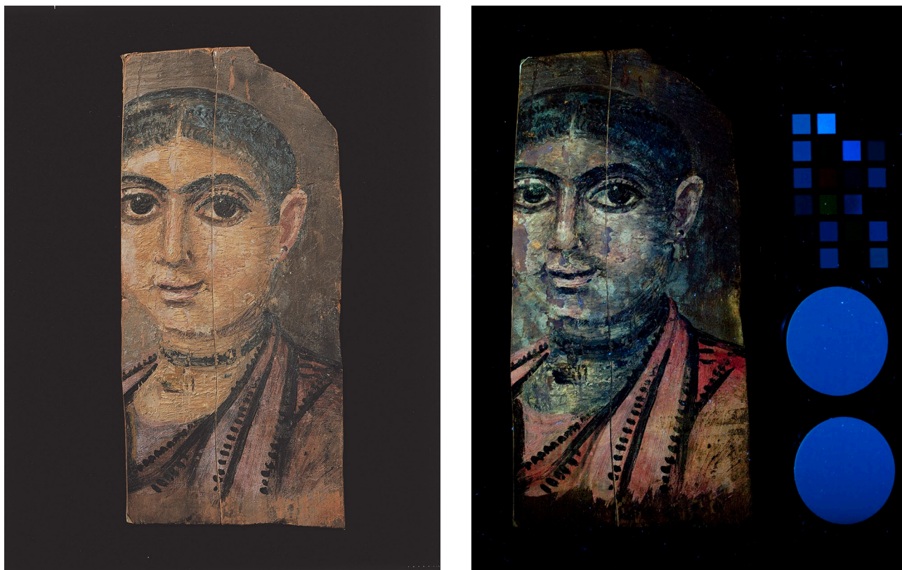
Fig. 11: Ultraviolet fluorescence (UVF) imaging can detect organic luminescent materials such as lake pigments, and is often used for the examination of mummy portraits. Left: Mummy portrait of a young woman, 2nd century AD. Ny Carlsberg Glyptotek, inv. No. ÆIN 682. Right: UVF image showing the orange-red fluorescence indicative of an organic red lake (photos: Maria Louise Sargent).
