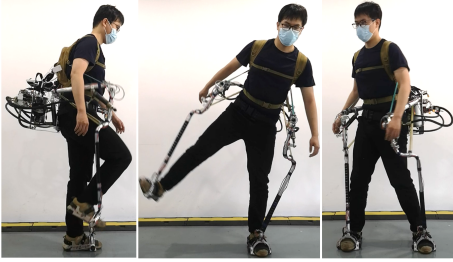
Fig. 10. The 6-DOFs of HyExo is demonstrated in motions such as stepping, abduction of the hip, and waist twisting.
