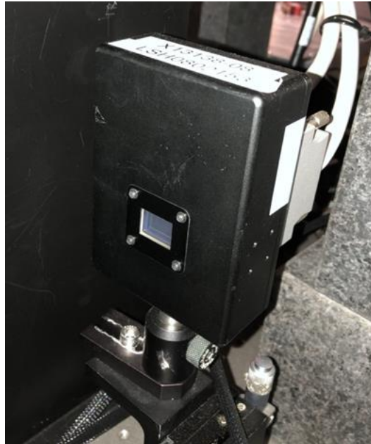
Fig. 25. A photograph of the Hamamatsu spatial light modulator, mounted and positioned within the final beam shaping assisted ULI system.
