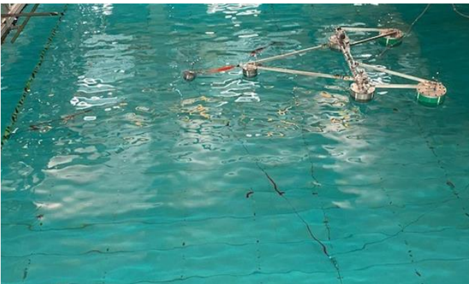
Figure 7: A photo of the layout of the M4 WEC and its mooring system in the wave basin
