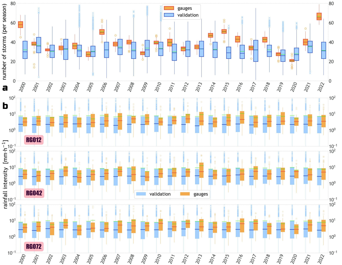
Figure 6. Yearly box-plots for the validation (blue), and gauge (orange) datasets. Panel a - Distribution of the number of storms in a wet season. Panel b - Distribution of storm intensities of three stations, i.e., RG012, RG042, and RG072 inside the Walnut Gulch catchment. In both panels, the green line within each boxplot represents the mean of the distribution. Please note the logarithmic scale of the y-axis in panel b (i.e., rainfall intensity). Supplementary Fig. B7 shows the (sparse) location of the aforementioned gauges.
