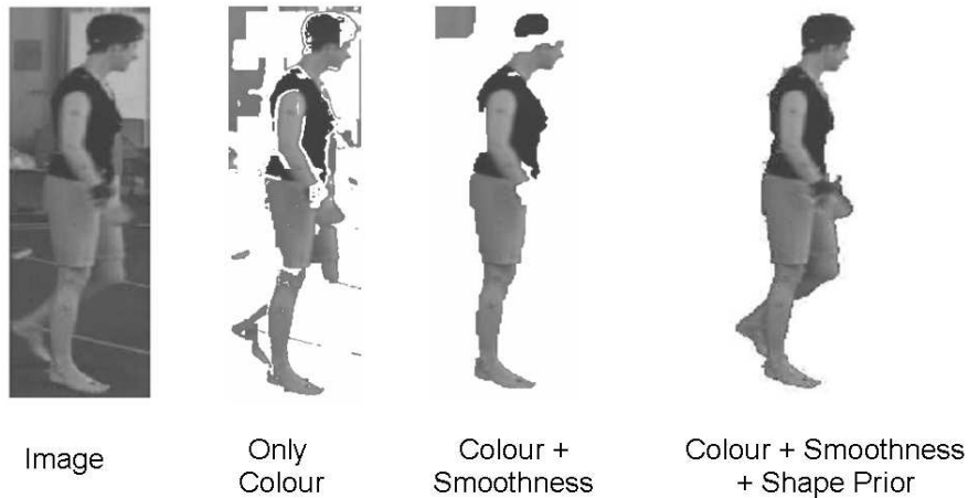
Fig. 8. Results showing the effect of incorporating a shape prior on the segmentation results. The first image is the original image to be segmented. The second, third and fourth images show the segmentation results obtained using colour, colour + smoothness prior and colour + smoothness + shape information respectively.
