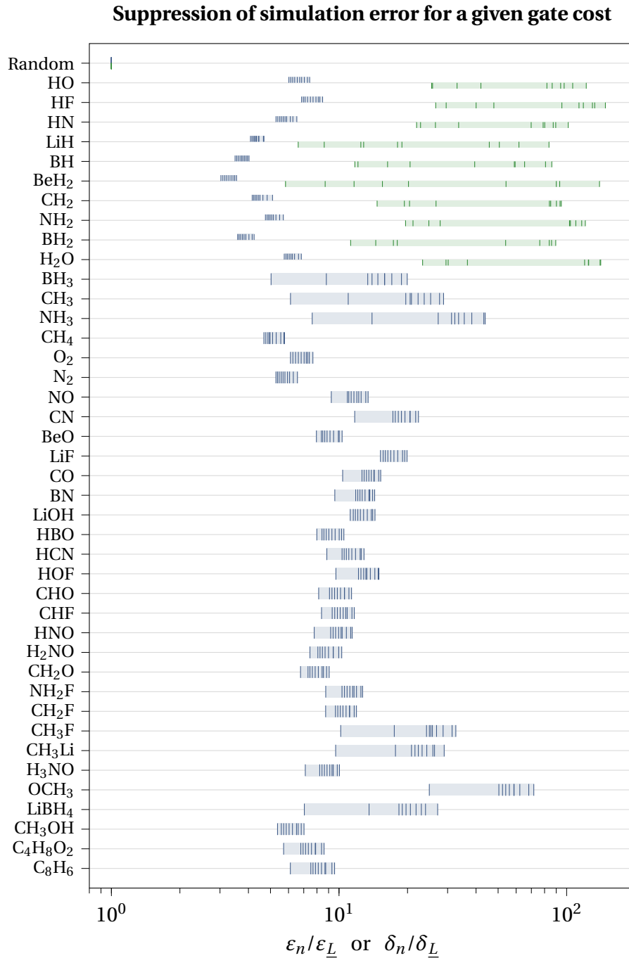
Figure 4.4: Magnitude of the errors obtained without, divided by the magnitude of the errors with the modification, for different molecules at identical implementation cost, using a time step of t_\infty . Errors were evaluated at cost values C_L = (1 \dots 10)L . Each vertical line represents the ratio of errors at some cost C_L , the shaded areas indicate the range from the smallest to the largest data point. The advantage of the modified algorithm therefore increases left-to-right. Top-bottom split data indicates ratios of error bounds \varepsilon_n/\varepsilon_L at the top (marked in blue) and ratios of numerically obtained errors \delta_n/\delta_L at the bottom (marked in green). If there is no split, the blue lines represent error bounds only.
