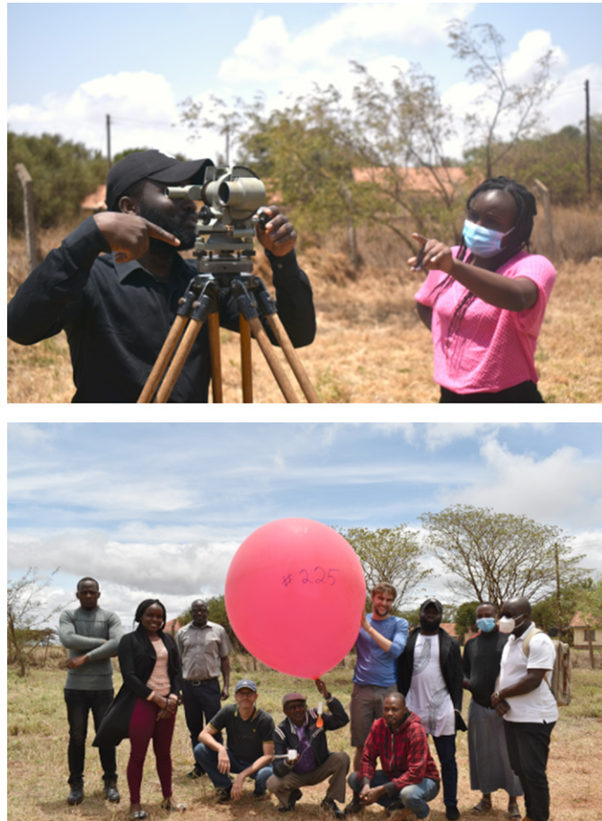
Fig. SB1. (top) Pilot balloon tracking using Kinuthia's theodolite. (bottom) The RIFTJet team gathers for one of the final balloon releases.
