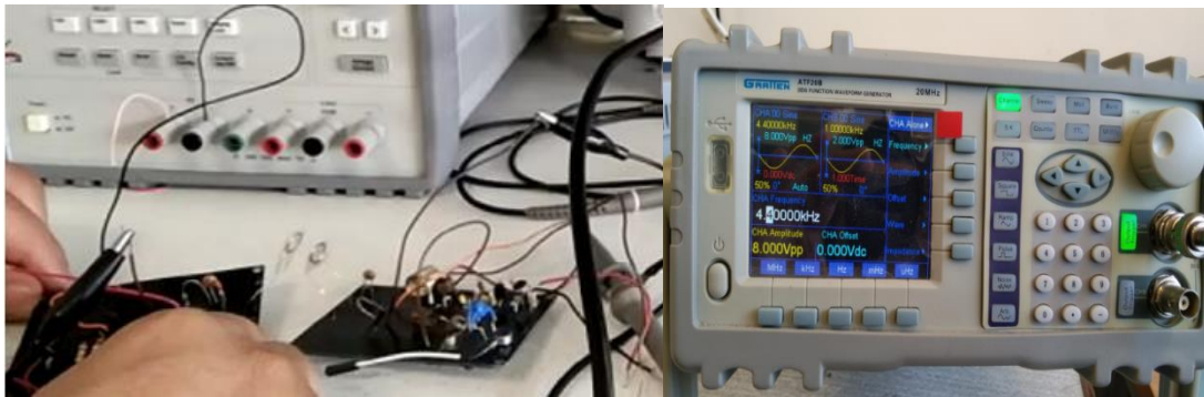
Figure 7 Experimental setup with tank circuits, device on the right was used to excite the primary coil
