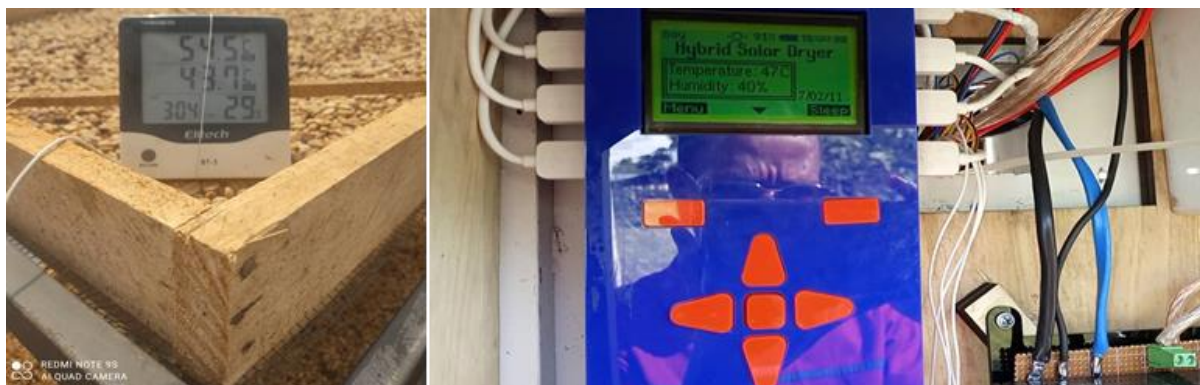
Figure 3. Monitoring relative humidity and temperature of coffee during drying using automatic sensor-based controls.
