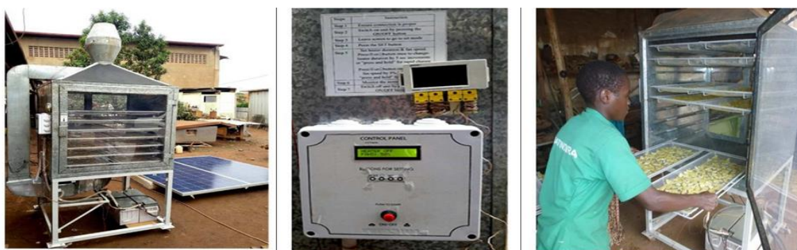
Figure 4. The major components of the Solar Photovoltaic and Electric (SPE) dryer [38].
