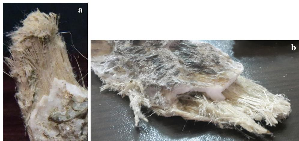
**Figure 2.** Photos showing microfibrils in sepiolite (a and b).
