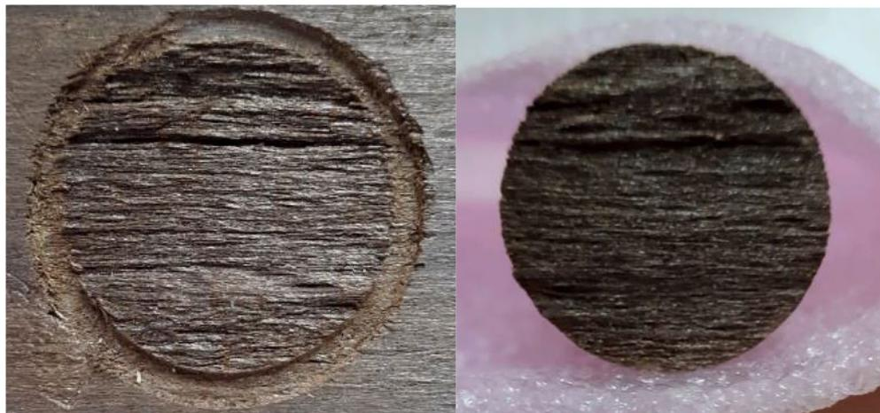
**Figure 7.** Pull-off specimen of the thermally-modified beech substrate illustrating full and accepted failure in the body of the wood substrate (no failure occurred in the adhesive layer) (magnification  $\times 2.5$ ).
