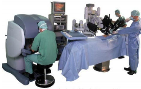
Figure 1. The da Vinci robotic surgery system
