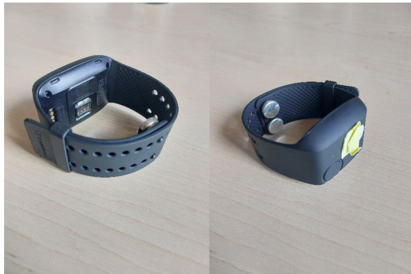
Figure 5. Empatica E4 smartwatch collects physiological data in the form of EDA with sensors seen from two perspectives of the device.
