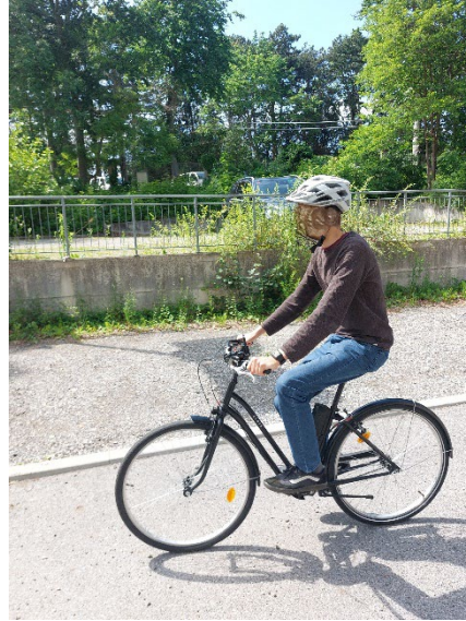
Figure 4. Instrumented bicycle with a smartphone attached to the handlebar and E4 smartwatch on the wrist.
