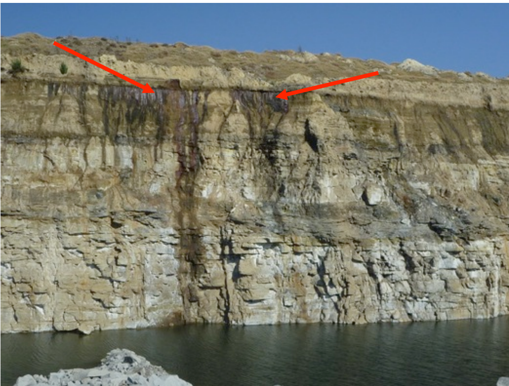
Figure 19 Opencast mine profile indicating a distinct flow path (arrow) beneath the soil profile
