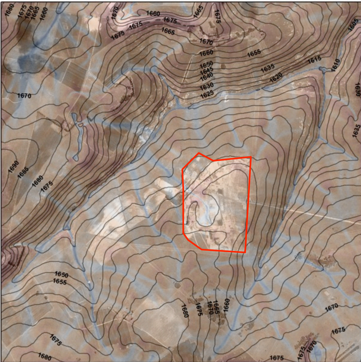
Figure 51 Position of the Jaglust mine (red polygon) relative to the two drainage features on the western and eastern side as well as the drainage depressions from the crest
