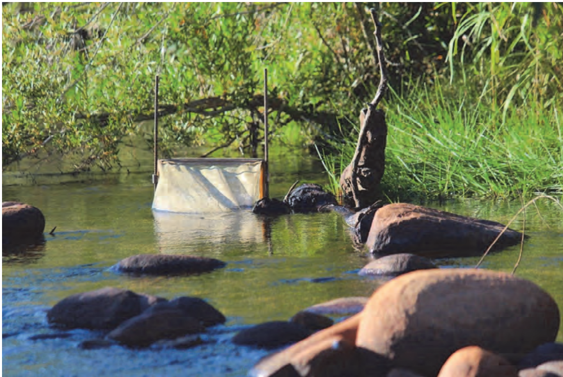
Drift net set up in the Rondegat River to collect invertebrates
