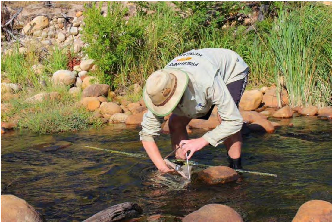
Researcher Darragh Woodford collecting stones into a 20 \mu\text{m} mesh net
