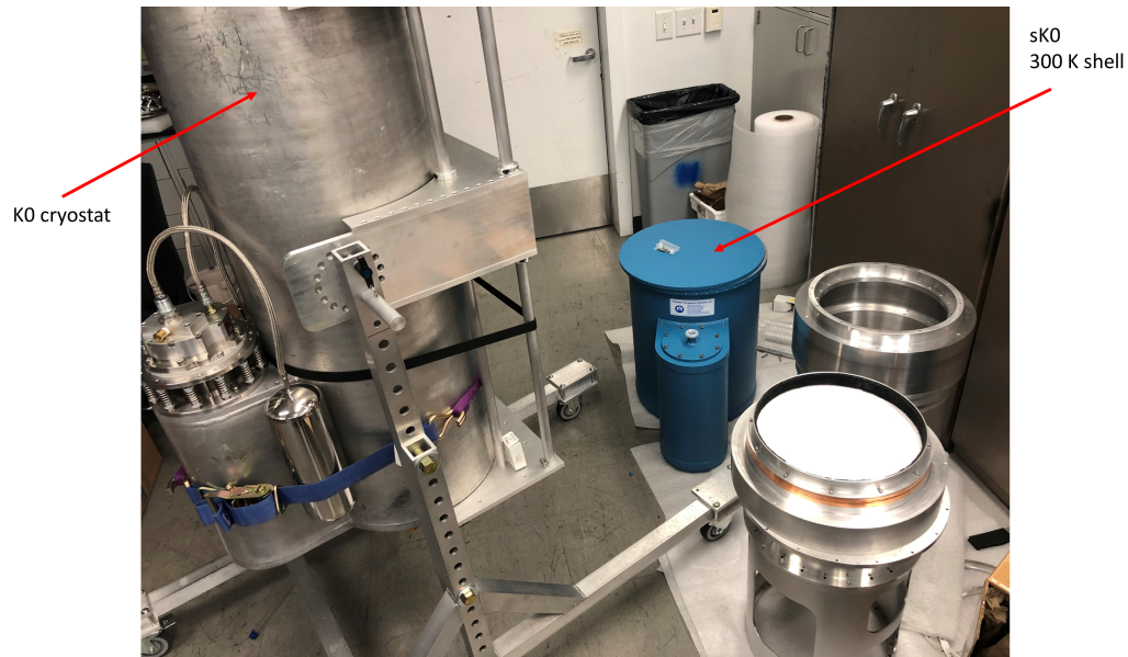
Figure 3.4: Picture of the unpacking of the sK0 shells. The K0 cryostat (in grey) is much taller than the sK0 300 K shell (in blue). We designed the sK0 shell so that we could access the UC volume of the cryostat without having to fully disassemble the telescope. The implementation of this new mechanical assembly led to a much faster testing turnaround time, from 10 FTE minimum to 1.
