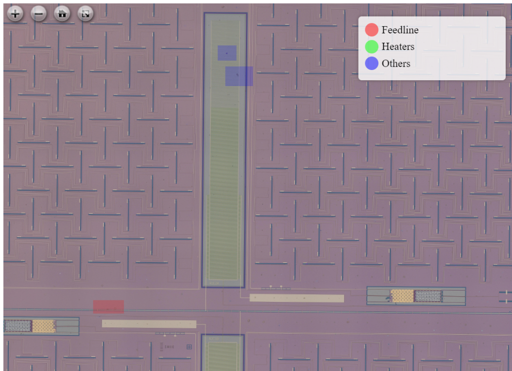
Figure 2.8: Web software interface displaying the buttons to draw rectangles on a tassalized images. Each color corresponds to a kind of defect. The category of the defect does not reflect any specific layer but rather the effect of the defect on the functionality of the array. A feedline problem cannot be ignored. A heater problem can potentially be ignored if fixing it would risk creating feedline problems. All the other problems, in blue, do not affect more than one device and can potentially be ignored. The user can pan and zoom freely, the backend records the absolute position of the box respect to the tile center and builds a report. In this specific screenshot we can observe two defects on the capacitor (blue boxes) and one on the feedline (red box). In the screen we can clearly see two islands (yellow patches) and the patterning of the dual polarization slot antennas (horizontal and vertical blue segments). A page taken from such report as an example is available in Figure 2.9.
