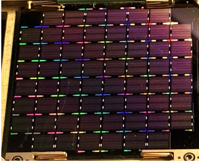
Figure 2.5: Picture of a TKIDs tile (receiver side) mounted to the FPU. The islands containing the inductive elements are visible as the iridescent small rectangles; the dual polarization antennas are the bigger squares. The 8x8 grid is clearly recognizable and so is the absence of the corner antennas. The 8 corner detectors do not have an antenna by design and are referenced in this work as dark devices. The tile is held in place via four Beryllium-Copper cantilever clips.
