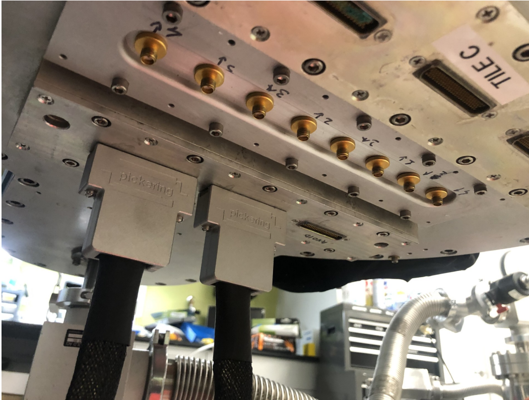
Figure 3.7: Bottom plate of the cryostat with custom housekeeping cables connected. Two 100 way cables are sufficient to operate the cryostat and diagnose most of the cryogenic problems. A third slot on the same plate is left unused. In the picture the RF front-end plate is visible (central) sporting 8 SMA RF connectors. An additional housekeeping-like plate is visible with the label “Tile C“. This last plate is used to route the calibration signals for the TKIDs array.
