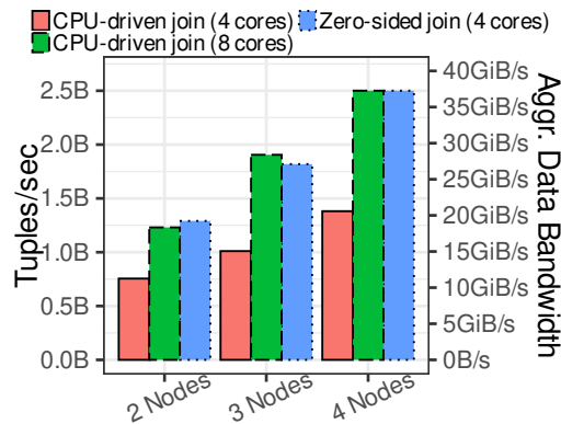
Figure 12.15: Distributed Join. Tables are shuffled from CPU-based storage nodes to GPU nodes for joining. Zero-sided RDMA achieves better performance with fewer CPU cores compared to [123].
