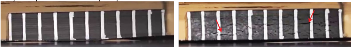
Figure 8: Deconsolidation of a specimen during heating, left image before heating, right image after heating with deconsolidation (cracks) at the red arrows
