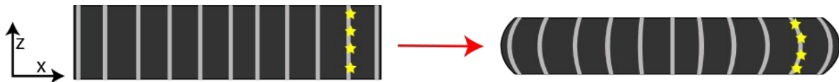
Figure 5: Points traced (yellow stars) on a line to obtain the local velocity during the squeeze flow of a specimen
